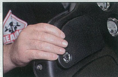
It's necessary to remove the fairing "clam shell" to install the speakers, which come with attractive covers containing tweeters.
